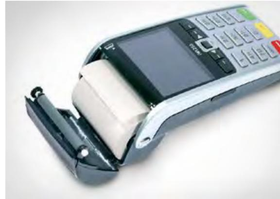
**2** Peel away the end of the new roll. Leaving the end free, hold the till roll and carefully place into the printer compartment.
