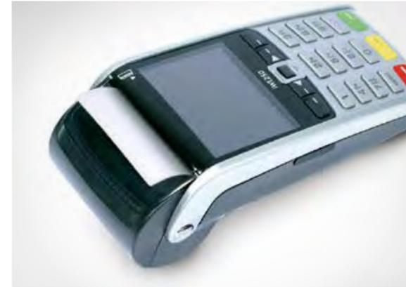
**3** Holding the free end of the paper and your card machine, close the printer cover carefully and push firmly until it locks.
