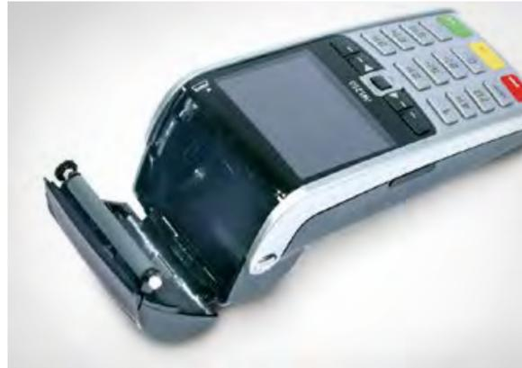
**1** Hold your card machine securely in one hand. With the other hand use two fingers to lift and release the printer cover.
